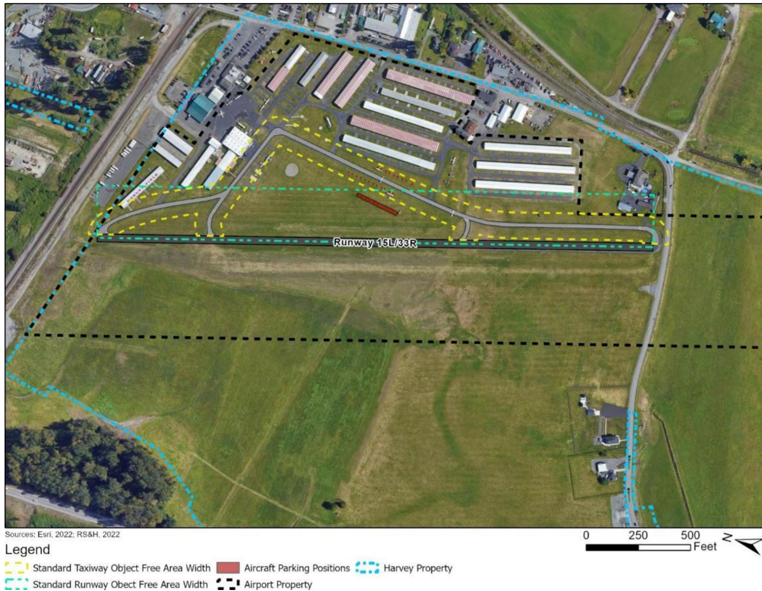
Figure 1-3 Runway 15L/33R Standard Runway Object Free Area and Taxiway Object Free Area and Existing Non-standard Aircraft Parking Positions
