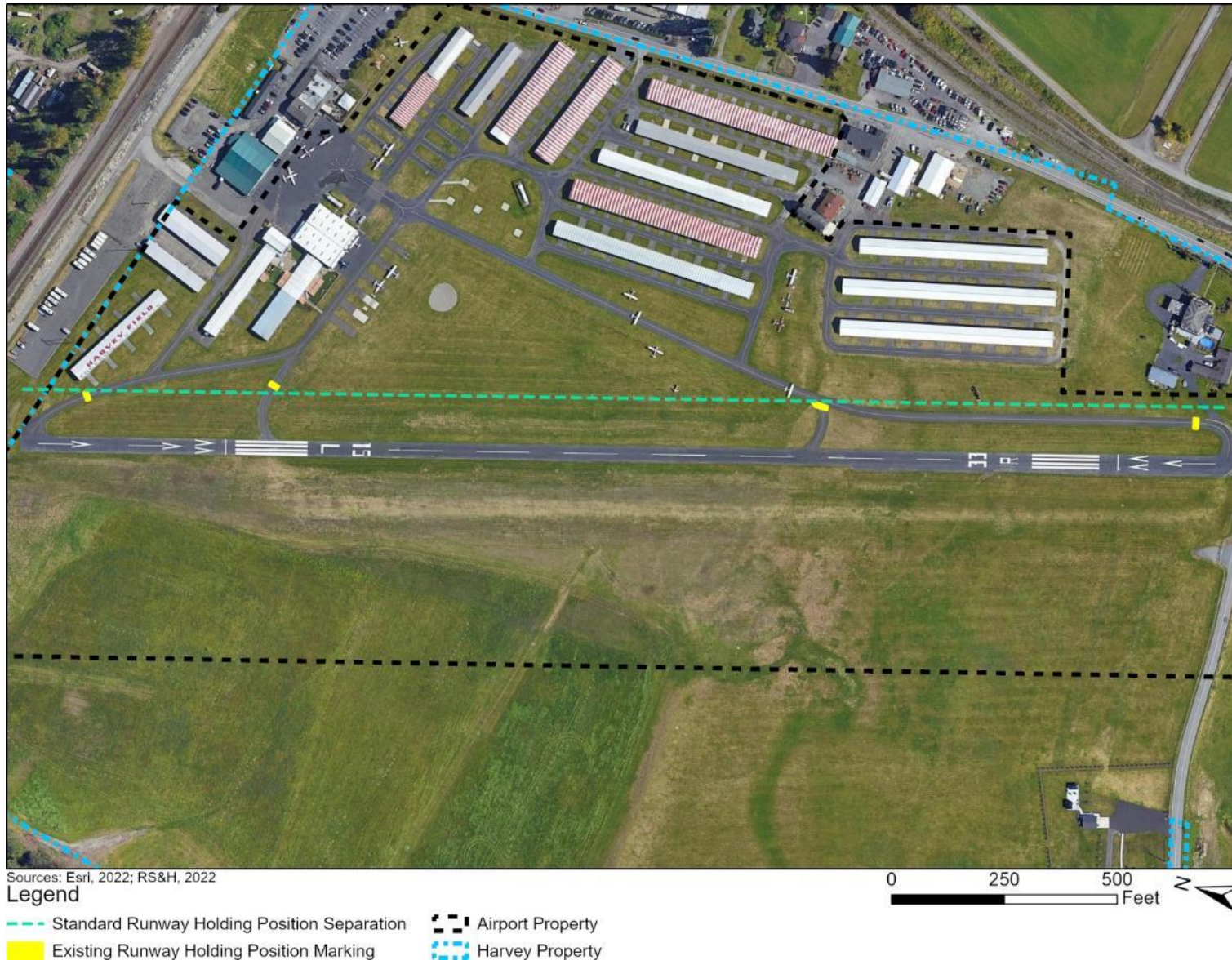
Figure 1-4 Standard Runway Holding Position Markings Distance and Existing Non-standard Runway 15L/33R Runway Holding Position Markings
