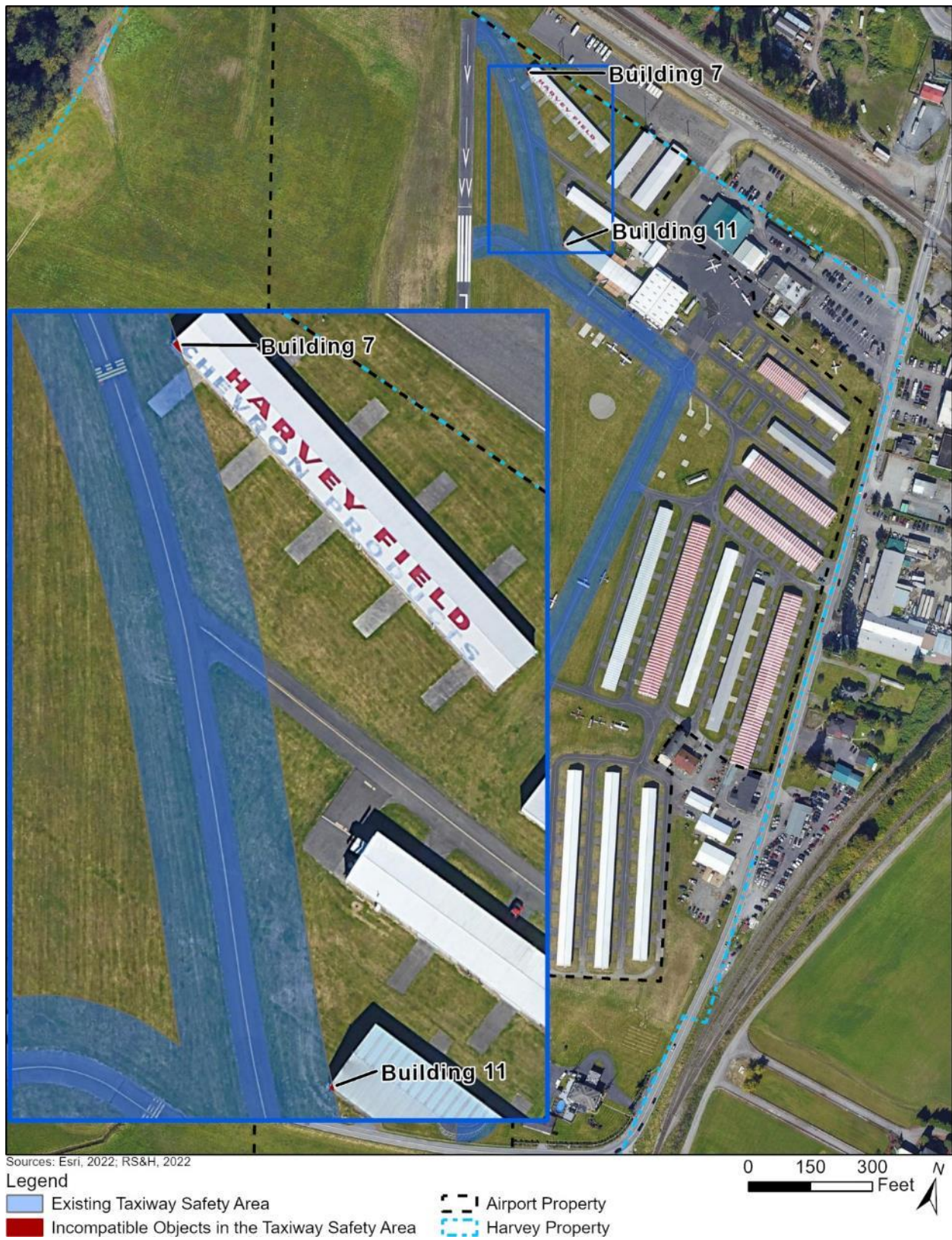
Figure 1-12 Existing Taxiway Safety Area with Incompatible Objects
