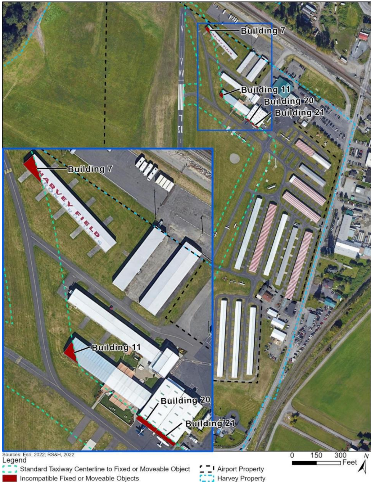
Figure 1-11 Existing Taxiway Centerline to Fixed or Moveable Objects and Non-standard Taxiway Centerline to Fixed or Moveable Objects
