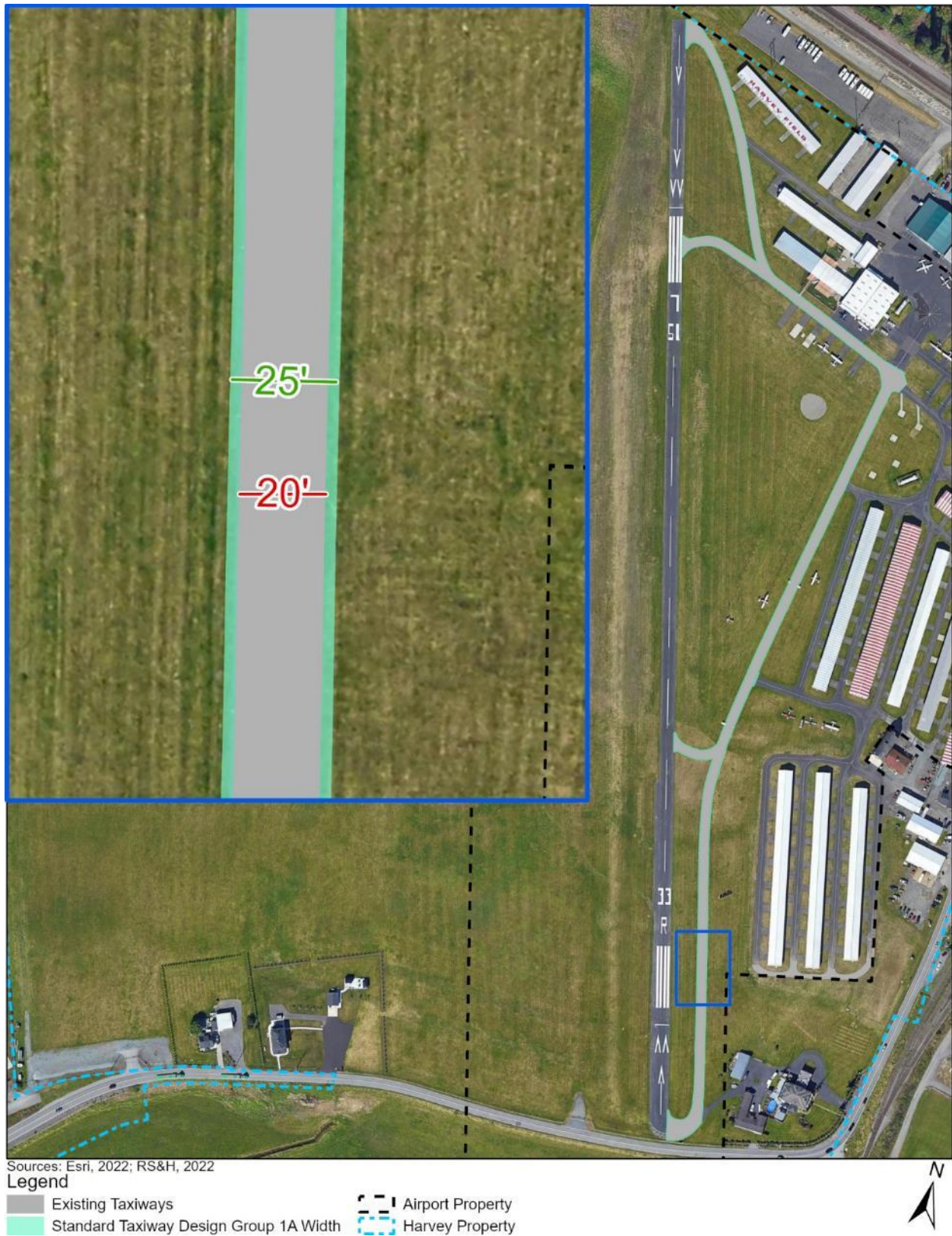
Figure 1-10 Standard Taxiway Width and Existing Non-standard Taxiway Width
